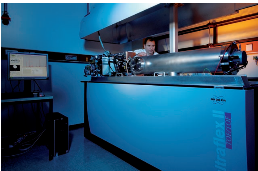
Figure 1: Peptide mixtures are identified in a single stage by MALDI-TOF/TOF mass spectrometry at the Fraunhofer IGB.
